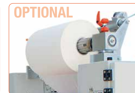
Ultra-fast film reel changer: It takes just seconds to load film reel thanks to its rotative expansible shaft system. This module includes a cutting wheel, which ultimately adapts the film width to the paper width.
